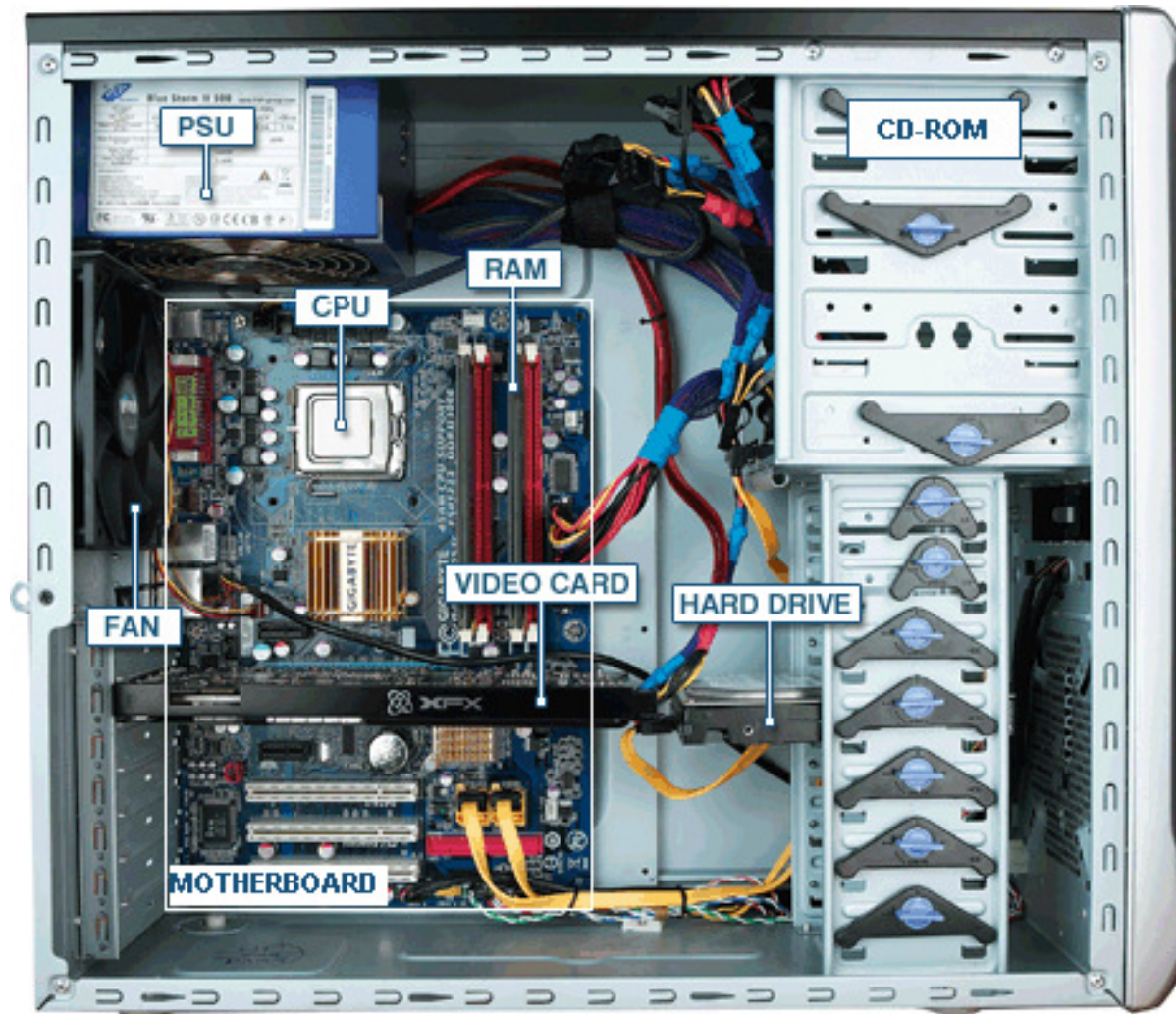
Basic parts inside a desktop computer
